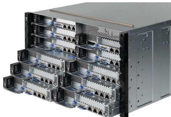
NeXtScale System comprises powerful compute nodes and an energy-efficient, low-cost 12-bay chassis.
